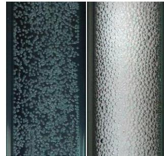
Bubbly flows at low (1.6%, left) and high (45%, right) void fractions.
