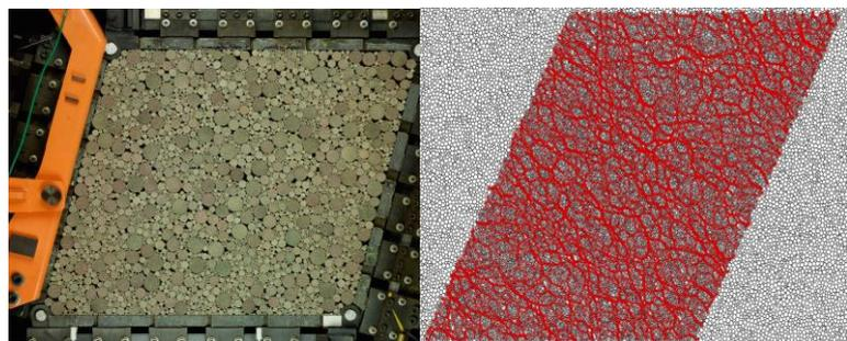
Sheared granular assembly of 2D grains –  $1\gamma 2\epsilon$  device (left). Sheared granular assembly of 2D grains and contact forces – DEM (right)
