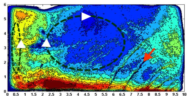
Solute composition map in a Tin-Lead alloy ingot solidified from the lateral sides. Digitalized X-ray image. Dimensions of the ingot 10×6×1cm<sup>3</sup>. The red color corresponds to the positive segregations.
