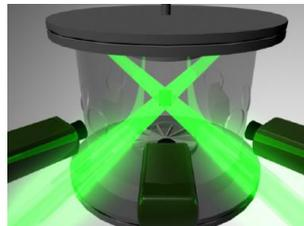
High resolution 3D Lagrangian particle tracking system
