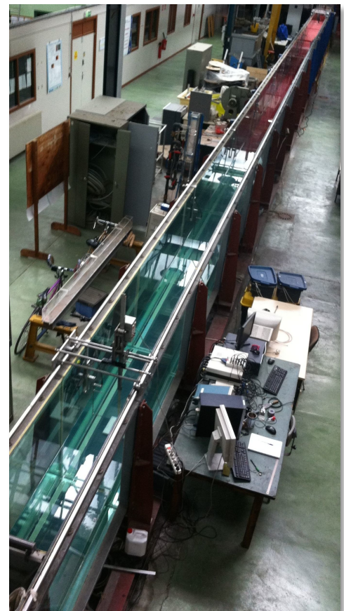
36m wave flume in LEGI. It will be adapted during the WATU project to study 1D wave turbulence.
