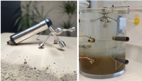
Figure 1: On the left, the three-component ADVP (Acoustic Doppler velocity profiler) prototype named UB-lab 3C, equipped with 1 central emitting transducer and four side receiving transducers. On the right, the cylindrical tank filled with tap water and natural estuarine mud.
