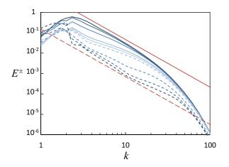
FIG. 4. (Color online) Energy spectra  $E^+(k)$  (solid line) and  $E^-(k)$  (dashed line) for the same five values of  $\eta_0$  as in Fig. 1 and the same color code. Increasing  $\eta_0$  the curves spread from the center towards the two (red) dashed and solid straight lines corresponding to  $k^{-7/3}$ .
