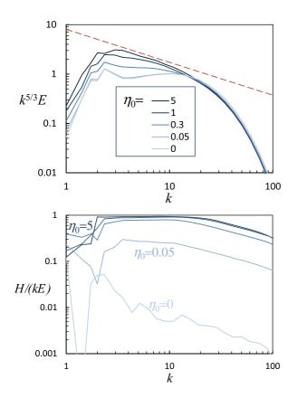
FIG. 1. (Color online) Spectral density of energy (top) and relative helicity (bottom), for five values of the helicity injection rate:  $\eta_0 = 0, 0.05, 0.3, 1, \text{ and } 5$ . In the top figure the energy is normalized by  $k^{-5/3}$  and the red dashed curve corresponds to  $k^{-7/3}$ .
