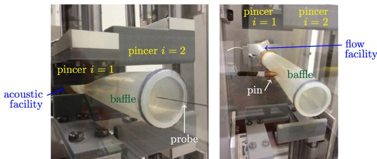
Fig. 1. Prototype of upper airway replica with a simplified time-varying waveguide set in a baffle. Both acoustic (left) as flow (right) fields are studied.
