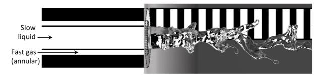
Numerical simulation of coaxial air-blast liquid atomizer. Low velocity liquid is issued from the round middle pipe, while a high velocity gaseous annular co-flow is injected around it, promoting liquid break-up. The image illustrates the type of behavior expected from the liquid jet.
