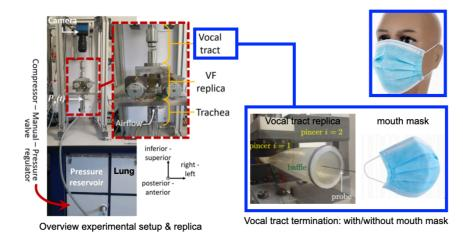
Fig 1: Overview of experimental setup and replica structure [1] and time-varying vocal tract [2] termination without/with mouth mask [3] to be studied.
