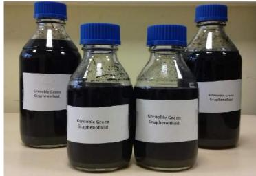
Graphenofluid containing SLG and MLG
