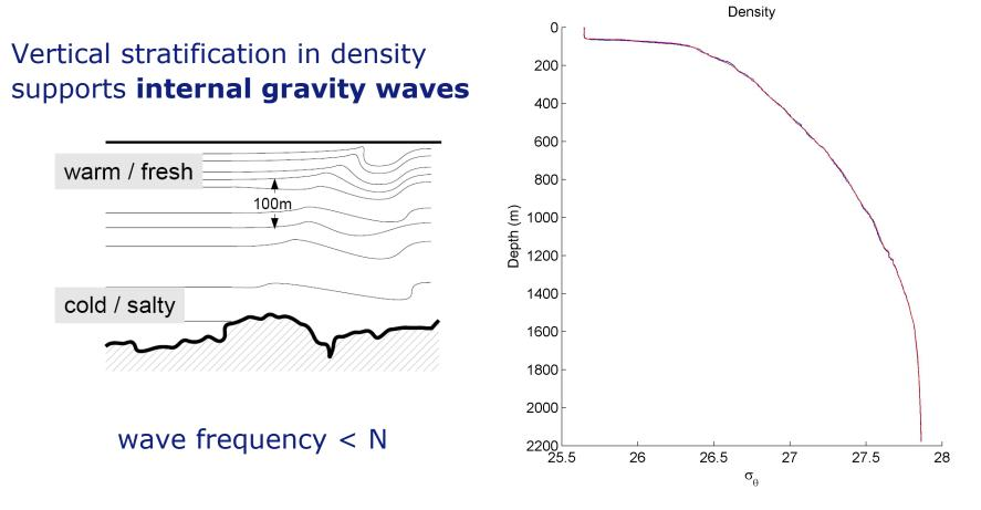
N = buoyancy frequency, function of stratification (=0 without stratification)
