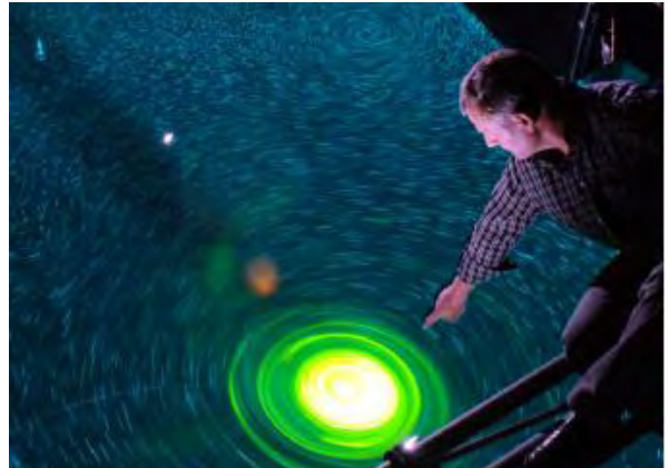
Vortex dynamics visualized by a laser sheet, used for combined Particle Imaging Velocimetry (PIV) and Laser Induced
