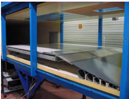
Figure 2. LML-AVERT ramp in the wind tunnel (left) and pressure distribution along the model for different flat plate angles.
