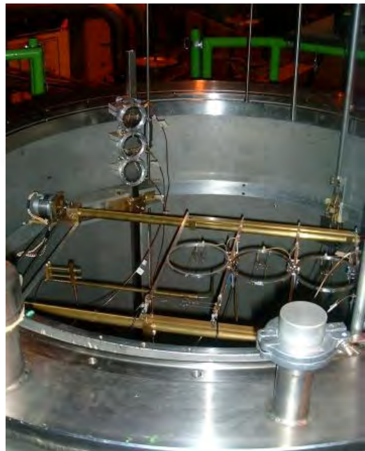
Left : Sketch of the GReC experiment. Right : picture of the inside of the jet chamber, with probes.
