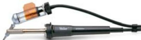
An 80 W/24 V desoldering iron for electronics rework. Electronically temperature controlled. Micro-finger switch controls quick-start, fast action vacuum pump. Different interchangeable tiptlets, plus several CSF devices are available as accessories. DSX 80 set, consisting of DSX 80 Desoldering iron, WDH 30 Safety rest, cleaning tool, glass collector, two desoldering nozzles, gasket, anti-bloc paste, filter.
