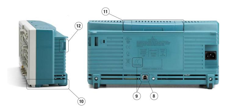
8 USB Device Port Combined with OpenChoice® and NI SignalExpress® TE for Seamless PC Connectivity – Easily communicate with other instruments, peripherals or systems via USB or GPIB (optional). The USB device port allows you full programmable control for automated measurements and remote display and archiving.
