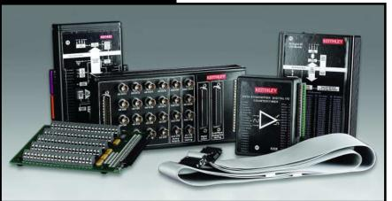
The Keithley KUSB-3100 Series brings true plugand-play data acquisition to computers that contain Universal Serial Bus (USB) 2.0 and 1.1 ports. No more opening up your computer chassis to install boards—just plug in the module, install the included software, and you are ready to
