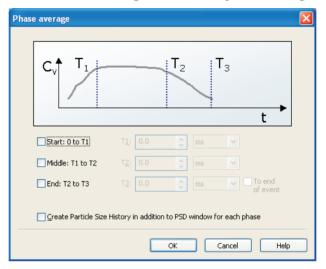
**Phase averaging** is generally used with single shot spray systems such as nasal sprays. It produces the averages of the start (formation), middle (fully developed) and end (dissipation) phases of a single event. The averages produced are stored as .psd files.
