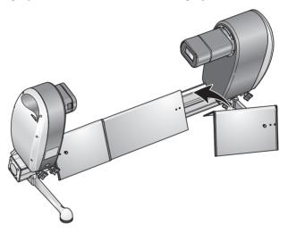
The shroud has three similar sections which clip onto the X-bar using clips on their lower surface. The central section has four clips, the others have two.
