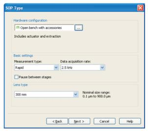
Click the **Hardware configuration** button and select **Open bench** with accessories. Keep the **Basic settings** measurement type **Rapid** and the maximum **Data acquisition rate** (2.5 kHz). Click **Next**.
