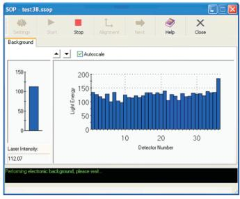
■ The instrument checks its alignment between the electrical and optical background measurements. If this is the first alignment in this session this may take some minutes, otherwise just a short time.
