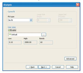
User size bands control the way data is aggregated; Chapter 6 has details. To use a different set of bands, select the **Enable** check box and click the button; Chapter 6 details the procedure.
