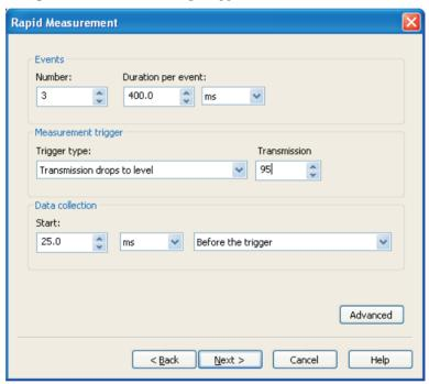
Set this up as shown above. This produces three 400ms events triggered by transmission falling to the 95% level, with data collection starting 25ms before the trigger condition is met.
