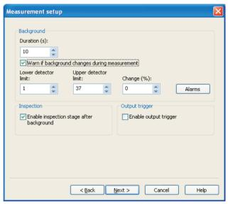
■ Use the **Duration** box to specify how long the background measurement will run for before moving to the next measurement stage.
