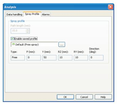
Default spray profiles for free spray and spray nozzle are provided. The parameters for the selected profile are displayed in the dialogue as shown above. Additional profiles can also be set up; these will be made available to other users at the site.
