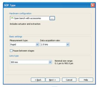
Click the **Hardware configuration** ... button and, if an actuator or extraction is being used, select **Open bench with accessories**. Otherwise just select **Open bench**. Under **Basic settings** the measurement type will be **Rapid** and the **Data acquisition rate** 2.5kHz. Click **Next**.
