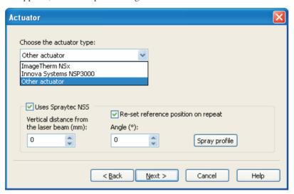
If using a Spraytec Nasal Spray Support (NSS), select the **Uses Spraytec NSS** check box and specify its setup; the online help gives full details. The **Spraytec Accessories manual** describes the NSS.
