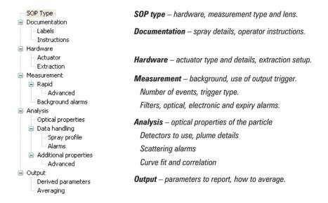
When an existing SOP is modified, this tree is shown to allow quick access to any of the dialogues.
