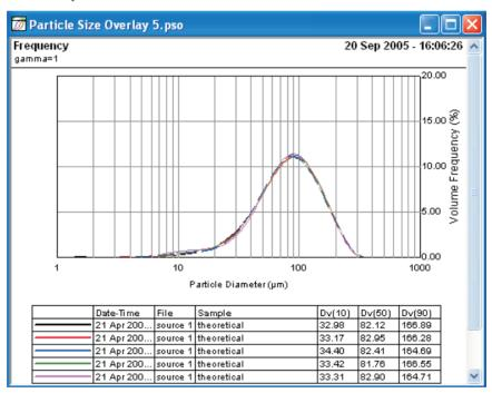
The table below the graph is a key to the lines and point symbols used and shows summary information for each file. Each data element is assigned a unique line style and colour; to change this follow the procedure below. To reformat the table, right-click on it.
