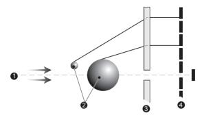
This diagram shows a parallel light source ①, particles of different sizes ②, the focusing lens ③ and the detector array ④.
