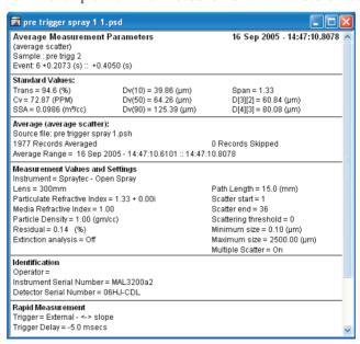
The window shows the same set of parameters as the Measurement Parameters window, but as averages for the range of records selected. This can be the whole measurement or a subset of records; the online help shows how to select a range and calculate averages.
