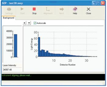
■ The **Laser intensity** is the non-scattered light measured by the Receiver. The example above shows this for the electrical background.
