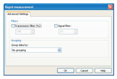
The **Transmission filter** removes results that exceed the indicated transmission level. The **Signal filter** excludes data signals that are below the indicated signal level. The signal level relates to the average scattering signal recorded across the active detector channels.
