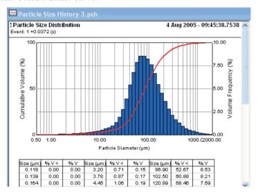
The histogram displays the result in the form of "in band" percentages. Each bar in the graph represents a size band of particles and its height represents the percentage of the spray that is within that size band. The user can edit the bands used.
