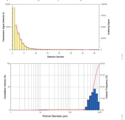
This spray contains a high concentration of propellant, causing a large scattering response on the first detector channels. This signal is much larger than the scattering response seen from the particles within the spray (detectors 30-35). As such the analysis reports a large particle mode, with only a small volume of fine particles being present.
