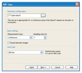
Click the **Hardware configuration** button and select **Open bench** as the hardware unless using extraction, in which case select **Open bench** with extraction. Under **Basic settings** keep the measurement type as **Continuous** and sample at one measurement a second or less. Click **Next**.
