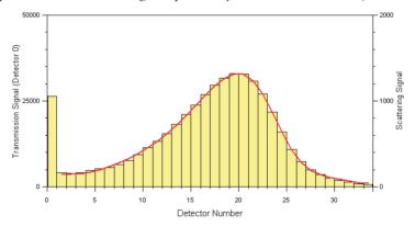
The detector array takes a snapshot of the scattering pattern. Note the following:
