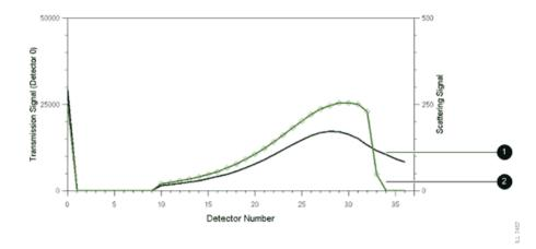
Curve ① shows the measurement made within the working range. Curve ② shows the measurement made outside of the working range. Here the lack of data on the last five detectors is obvious. This is caused by vignetting.
