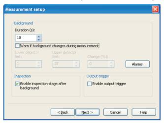
Select the **Enable output trigger** check box. This provides an industry-standard TTL trigger output for the control of other devices including accessories such as nasal spray actuators. This trigger is activated when the measurement starts and returns to its initial state when the measurement ends. Chapter 10 describes these triggers. Click **Next**.
