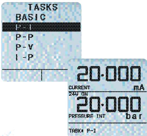
The **P-I** task configures the DPI 610/615 to simultaneously display the **OUTPUT** pressure and the **INPUT** current. The pressure unit can be chosen to suit the transmitter and a **24V** supply is available for loop power. (not IS version).
