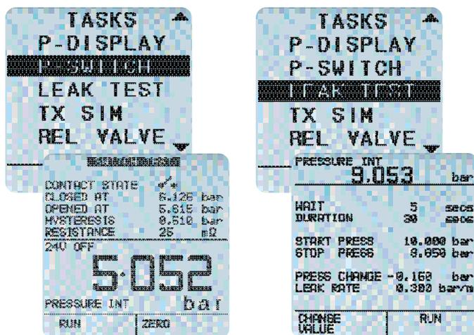
For Switch Set-up and Fault Finding, the display shows the output pressure and switch state **OPEN** or **CLOSED**. Continuity is declared by an audible signal.
