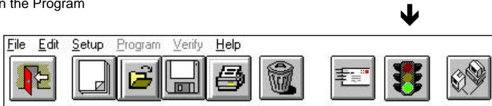
To run the program just sent, select the *Start Button* (Traffic Signal Icon Button) which signals Green for GO.
