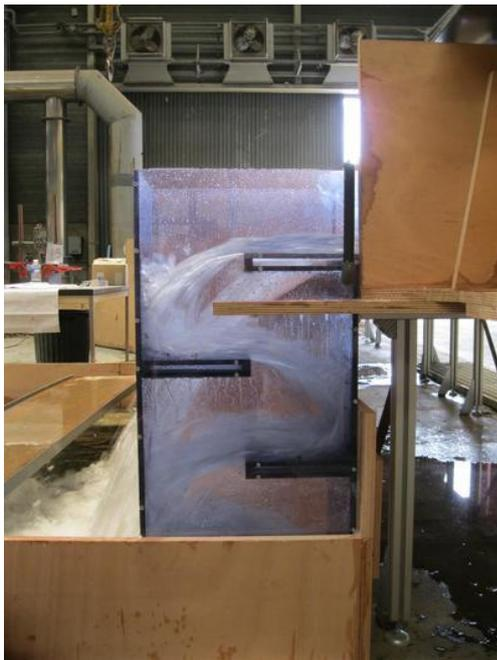
*Model of a bearing chute (Versailles, France) - Scale: 1/15. Experiments carried out at ARTELIA laboratory.
