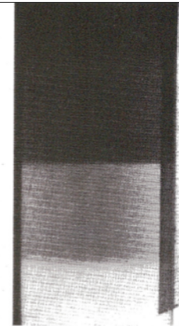
Fig. 8.8. (Left.) Vertical cross-section of salt fingers, marked by fluorescein dye added to the upward moving fingers, and lit with a thin sheet of light perpendicular to the viewing direction.
