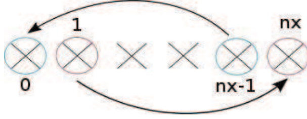
Figure 2: Scheme of the periodic boundary conditions in the x-direction
